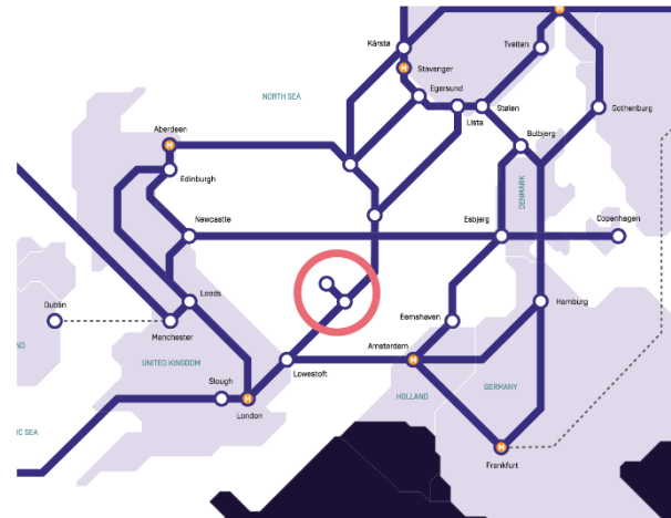
Figure 1: Tampnet fibre-cable network in the North-Sea. The red circle illustrates the use of a ROPA on the cable from the Valhall oil and gas installation, to Lowestoft in the U.K.
